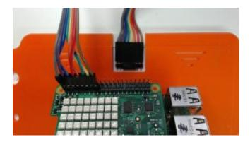
Note that Raspberry Pi with the Sense HAT can still fit in some cases like the Original Raspberry Pi 3 Case if you keep the top off.
