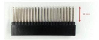
Don't worry if your header doesn't exactly look like the one in the picture, the important thing is that the metal part is at least 1.2 cm tall to allow for the Flick Large jumper cable to plug onto it.
