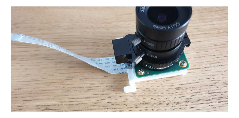
**Step 4** - Finally slot the adaptor with the camera module attached into the case. Make sure that it sits flush with the case and then slide it outwards to clip into place. We have provided a hole underneath to allow you to grip it form within the case.
