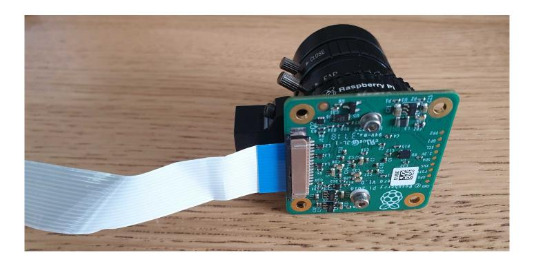
**Step 3** - Feed the camera cable into the available slot and then begin to screw the camera module into the adaptor.
