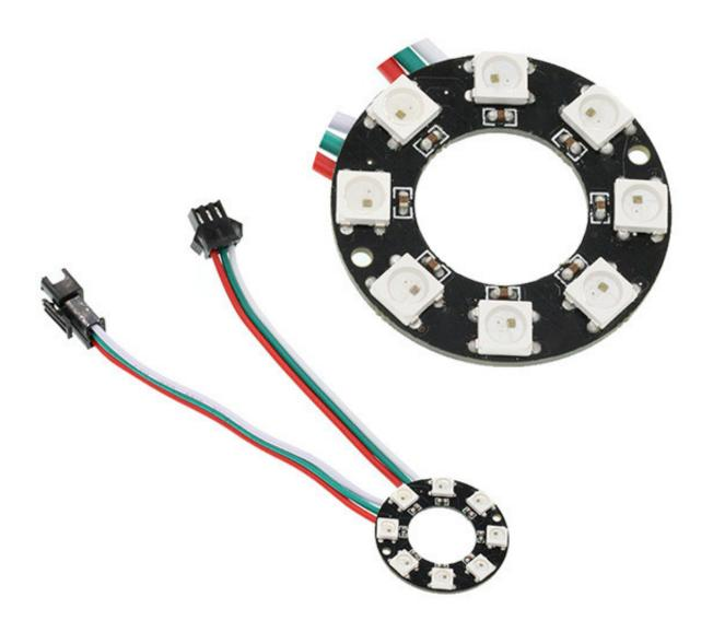
8 RGB Rainbow LED Ring is an LED ring made of 8 ws2812b LEDs in cascade connection. Ws2812b is an intelligent outer control LED source, which has integrated control circuit and light emitting circuit. It has same appearance with 5050 LED.
