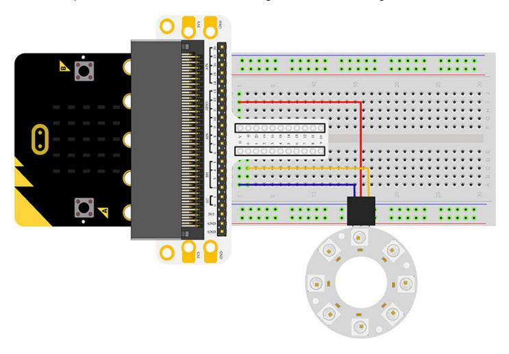
Note: There are two cables lead out by the ring. One is DI and the other is DO. We should connect DI.
