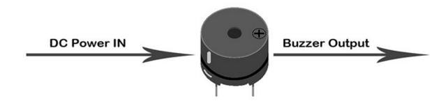
The working principle of passive buzzer is: When square wave signal pass through the buzzer, its resonance device will transform the square wave signal input into sound signal output. Below is the schematic diagram for the working principle of passive buzzer:
