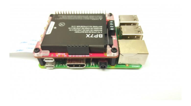
**Step 2.3** - Lastly, lets stack the Media Centre HAT. You will need to snap off the mounting holes on each corner first. You can do this with a pair of strong pliers and apply a fair amount of force to do this. Once snapped off mount the MCH HAT on top of the PiJuice HAT.
