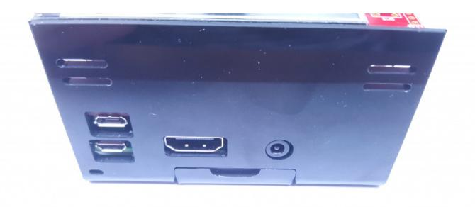
**Step 4** - Now take the top half of the case and carefully slide it over the bottom half making sure that it slides into the groves the are cut into the top half and it should just click into place.
