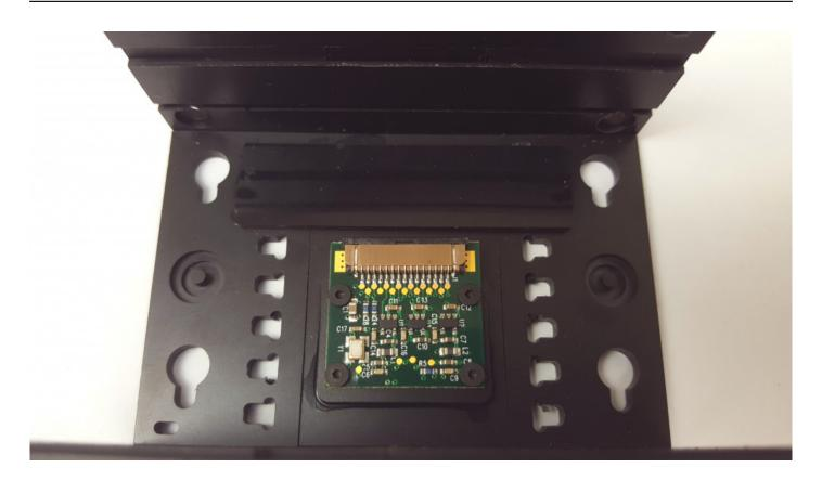
**Step 3.2** - Take the bottom half of the PiJuice Case and slot all the boards into it, making sure that you align the cut out holes in the side correctly with the correct connectors of the Pi and the PiJuice. The boards should then slot into the grooves on each side.
