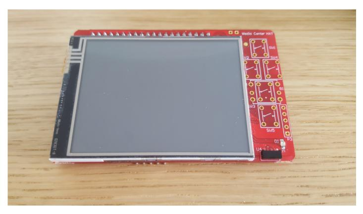
Step 2 - Now you can stack the Media Centre HAT on top of your Raspberry Pi, carefully inserting into the 40 way GPIO header.
