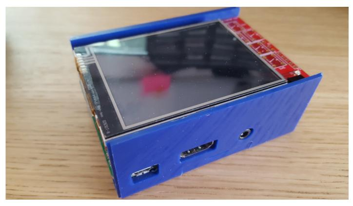
Step 4 - Take the top half of the case (Red) and carefully slide it over the bottom half, making sure that the drives slot in to the top half. Slide it over until it clips into place.
